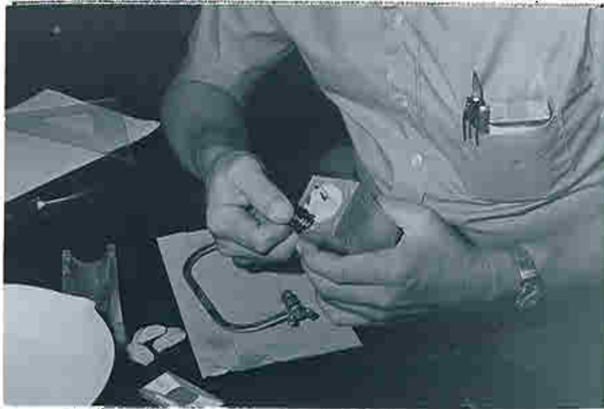
Figure 11. Sample placed in 8 cm miter box and cut to 8 cm length
