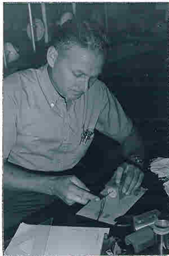
Figure 10. Insertion of a wet, double wool yarn, internal drain
